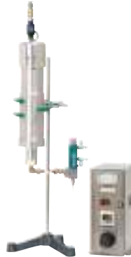
Cartridge-type tank Diaphragm type automatic valve Controller for pressure (coater SIII)
