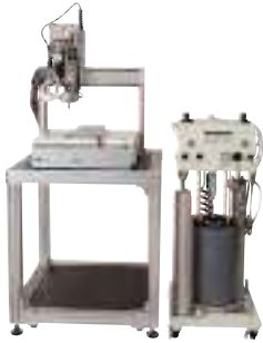
Pump for pails (PBIII-45) Constant-rate injection head (fixed-quantity booster) Desktop 3-axis robot (TRC-130N)
