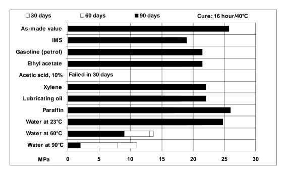
Lap shear strength versus immersion in various media at 23°C (typical average values)
