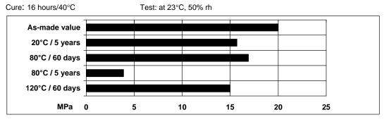
Lap shear strength versus tropical weathering (40/92, DIN 50015; typical average values) Cure:16 hours/40°C: Test at 23°C.
